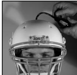
2. It is important to use a well-lubricated Schutt® Model 7790 Inflation Needle. Glycerine is recommended. DO NOT USE A PETROLEUM JELLY. Insert with a careful twisting motion making sure not to puncture liner's opposite wall.
